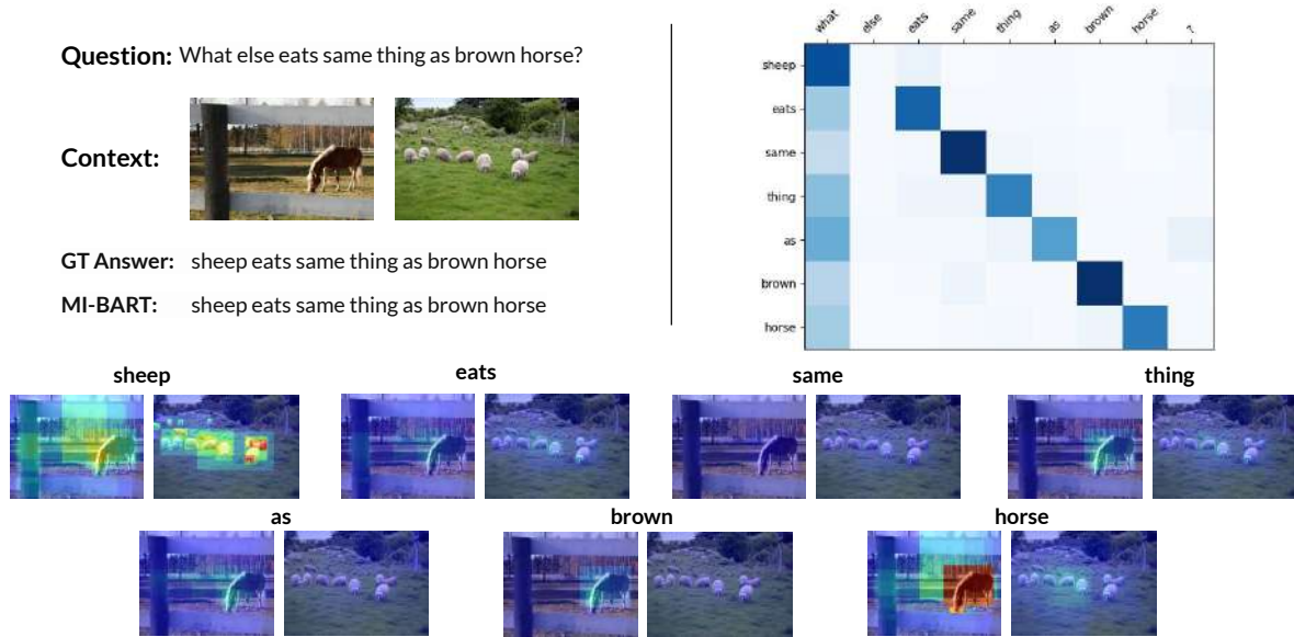
Figure 5.7: Multimodal attention map over the retrieved images and the question during the answer generation. We observe that our proposed MI-BART attends to the relevant regions of both images while generating the main answer word ‘sheep’. Further, we see that it attends to brown horse regions of the first image along with the corresponding question parts while generating ‘brown horse’. [Special tokens are removed for visualization.] (Best viewed in color).
